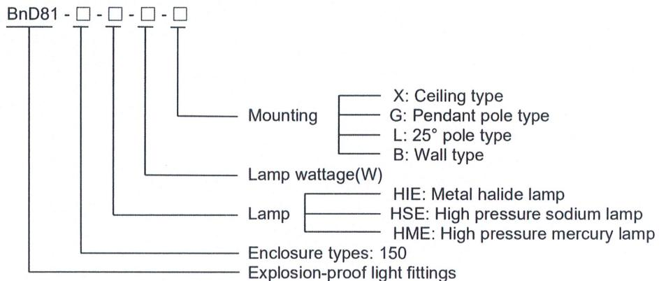
The options for lamp wattage are: 70W, 80W, 100W, 125W and 150W.
