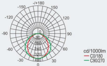
We can provide lighting design and data by professional lighting software DIALUX based upon simulated site situation on request.
